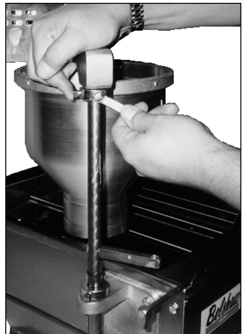
Figure 1-9. Adjusting the Swing of the Hopper.
