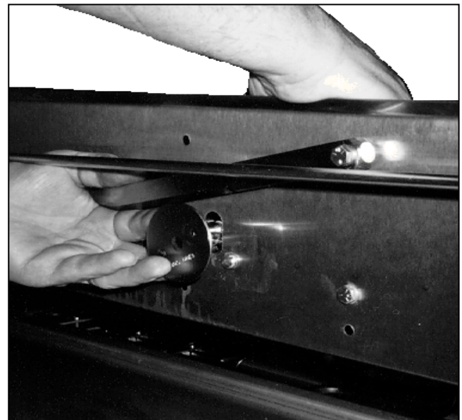
Figure 2-2. Removing the Turner Cam Assembly.
