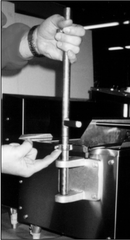
Figure 1-3. Inserting the Swing Column.
