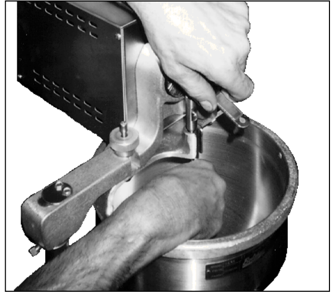
Figure 1-7. Installing the Plunger.
